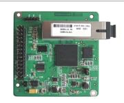
Remote Communication EPON ONU Module TP200C
